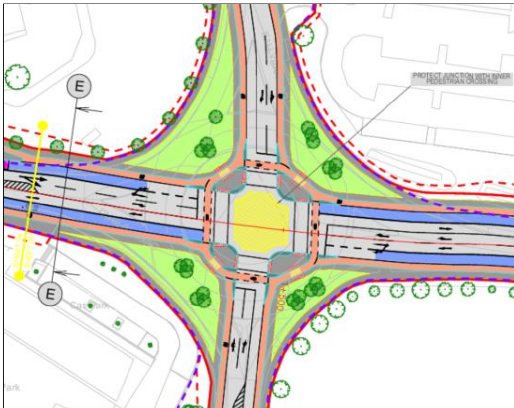
Figure 6-3 Skerritt Roundabout (Cyclops) Indicative Design
